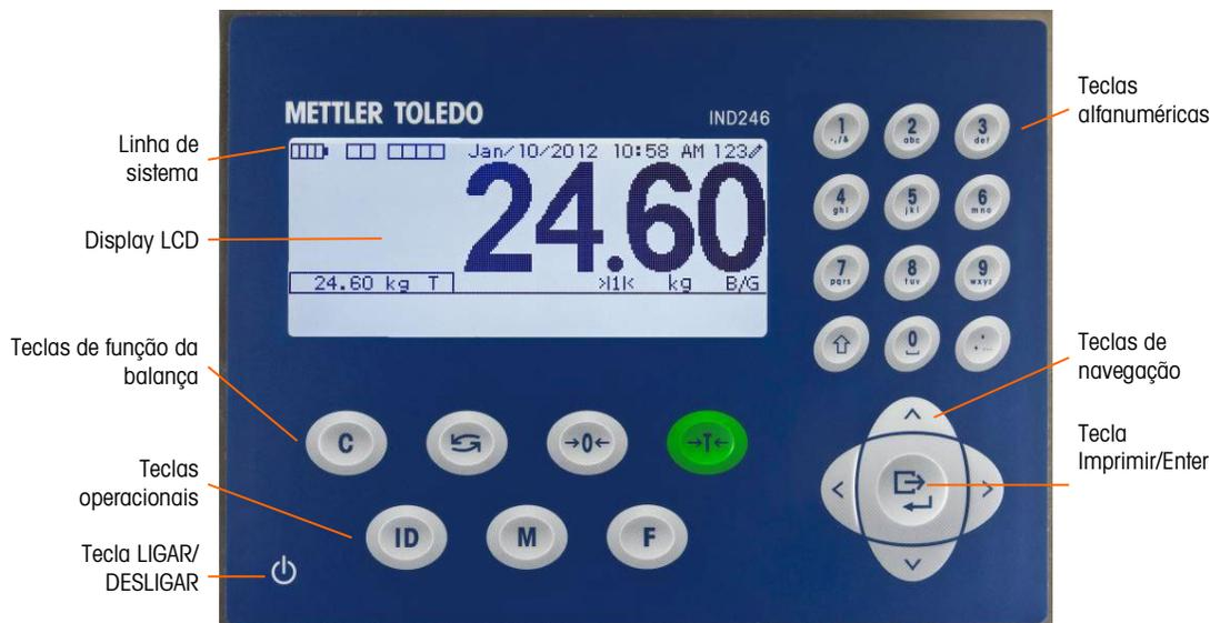
Figura 1-5: Layout de painel frontal IND246
