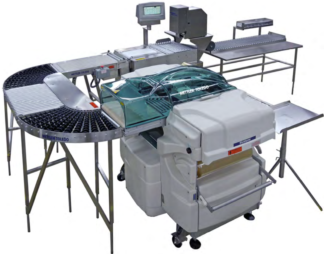
Workhorse® ZS with 90S90 Powered Conveyor and Model 707 Indexer/Labeler
