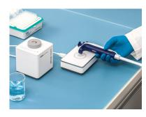
**Step 1:** Scan pipettes with an RFID reader or enter data directly.
